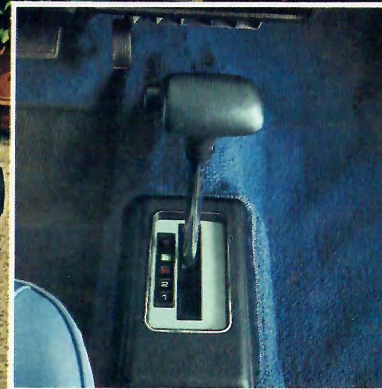
Hondamatic with torque converter and two manually selected forward speeds is an available option if you prefer clutch-free driving.
