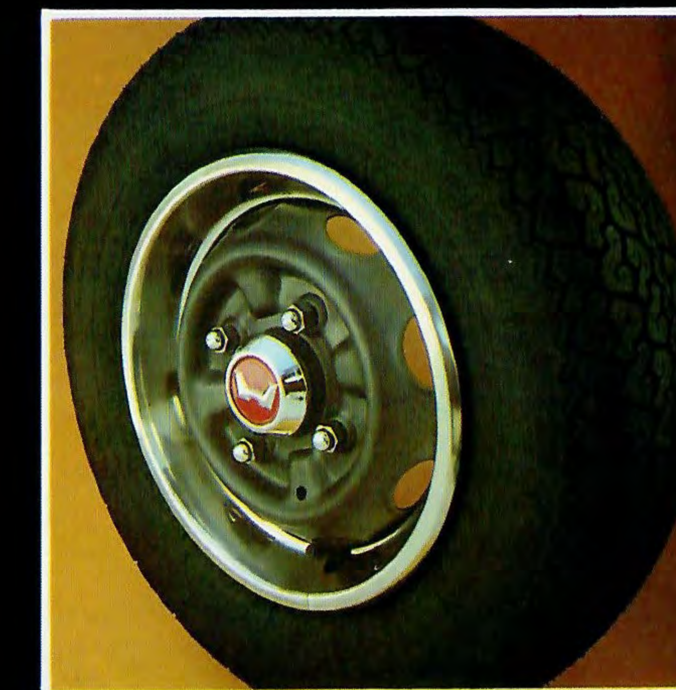
The Civic CVCC 5-Speed model has steel-belted radial ply tires and bright metal trim rings as standard equipment.
