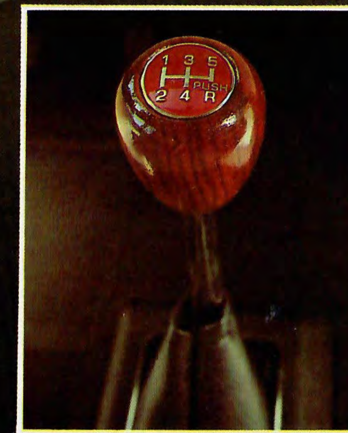
The 5-speed manual transmission provides a top overdrive cruising gear... saves fuel and engine wear and reduces engine noise level.
