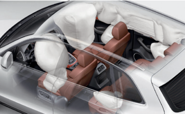
.26 – Six Standard Airbags With six standard airbags, including front-impact and thorax side airbags for both driver and front passenger, and available rear passenger thorax side airbags, you'll feel practically surrounded. 1 And that's a good thing.
