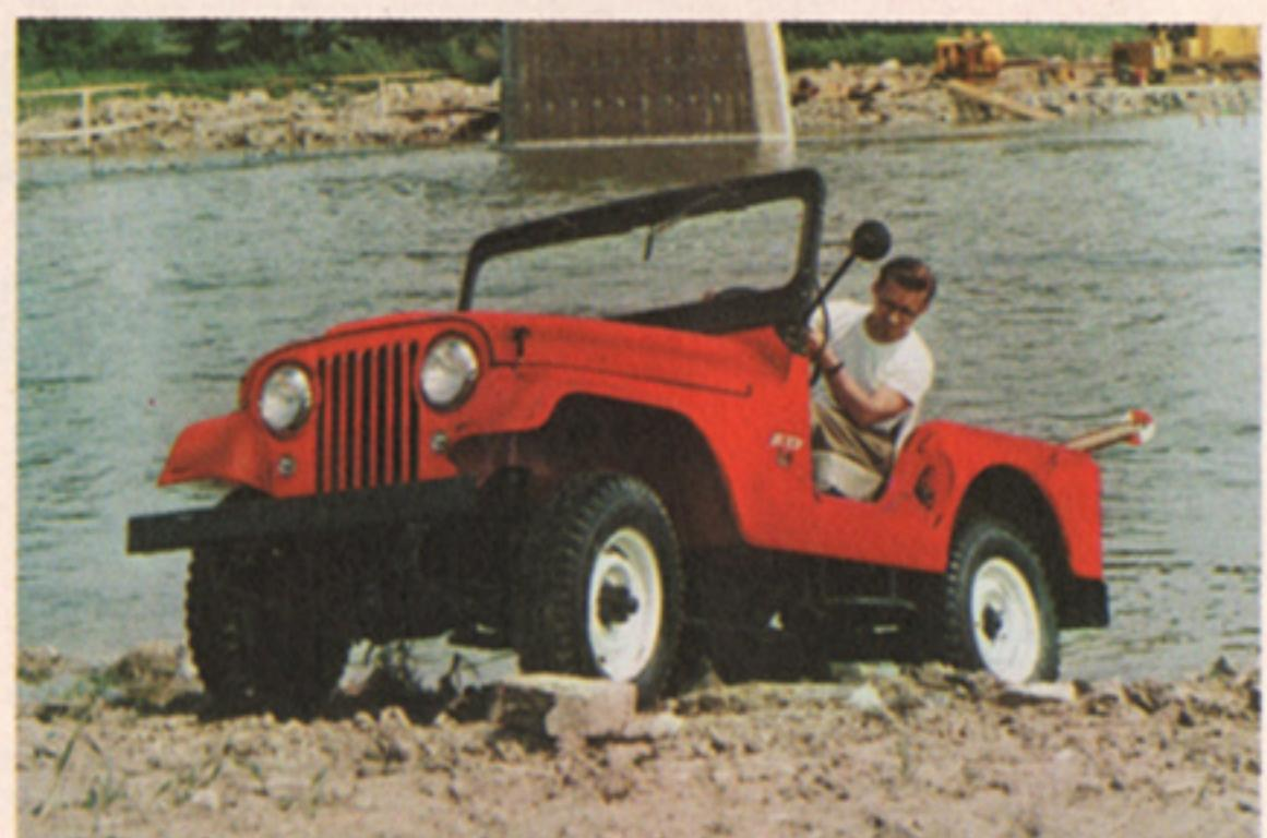
'Jeep' 4-wheel drive puts driving traction at all four wheels . . . provides safer going over wet, slippery roads—lets you drive over rutted trails and job sites where there are no roads. With its high ground clearance and short front and rear overhang, the Universal can pass over off-road obstacles and drive over hilly terrain. Four-wheel drive also provides for power take-offs to facilitate snow plows, winches, and many other equipment items. Payloads range up to 1564 pounds.
