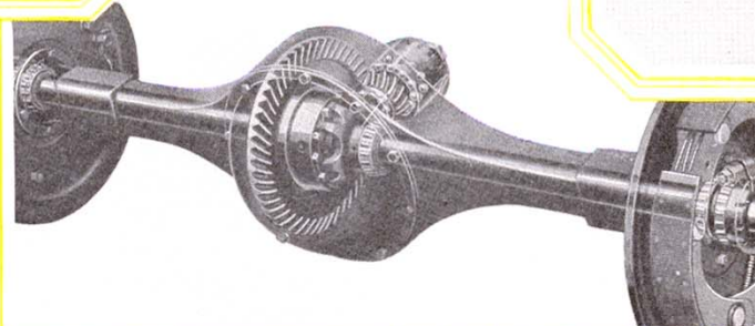
A "phantom" view of the special heavy duty rear axle—note the heavy box section housing and large shafts.
