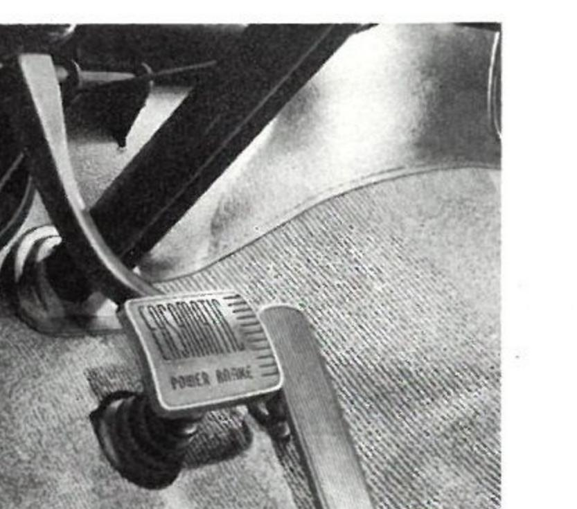
Pivot your foot—don't lift it. The low-level pedal is at the same convenient height as the accelerator—lets you apply brakes more quickly and safely.
