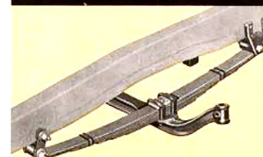
New, longer, wider front springs (F-100 and F-250) are more resilient for greatly improved truck riding qualities.
