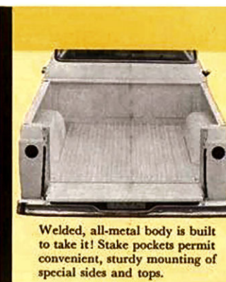
Husky box-like corner post construction combined with sturdy tailgate provides unequalled body rigidity.
