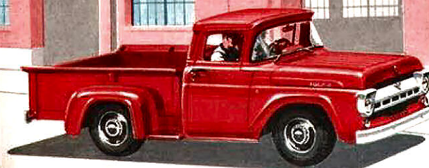
F-250 8-Foot Pickup (Shown with Standard Cab) Maximum GVW: 7,400 pounds Wheelbase: 118 inches
