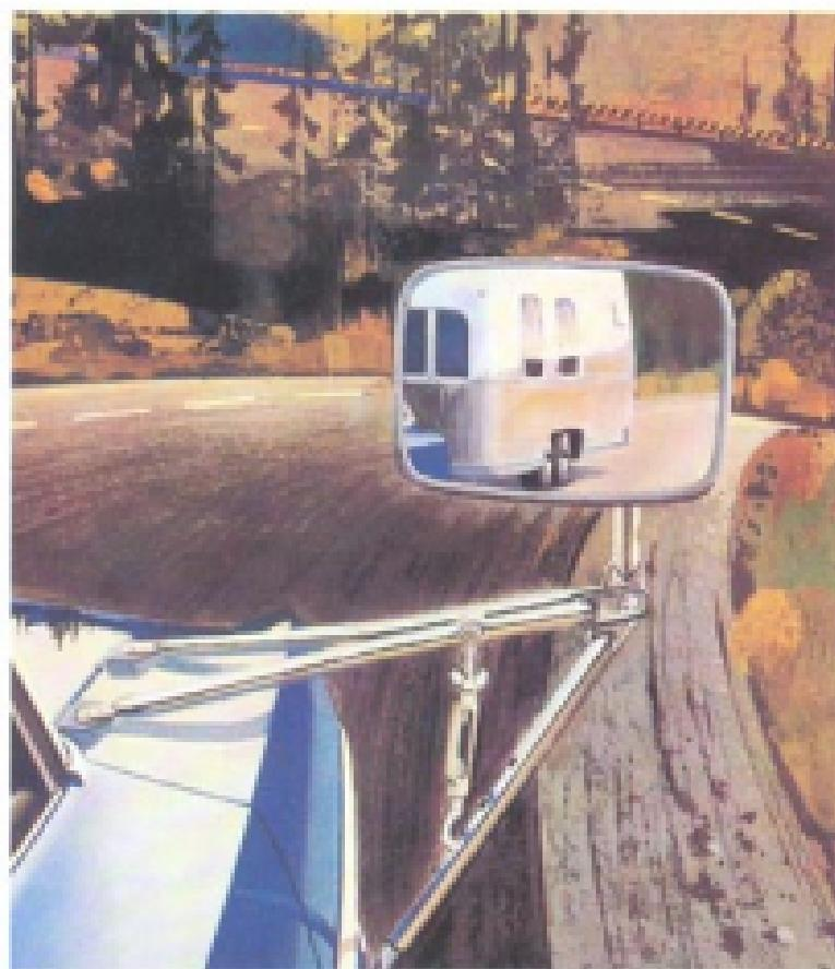
When you're towing a big trailer, conventional mirrors may not be enough. Help provide a good look at the road behind with a pair of specially designed Chevrolet trailing mirrors. They're big (6" x 9") so you get a large, clear view. Rigid clamping devices make installation easy and secure. And they're built to last, made of stainless steel and first-surface chrome mirror glass.
