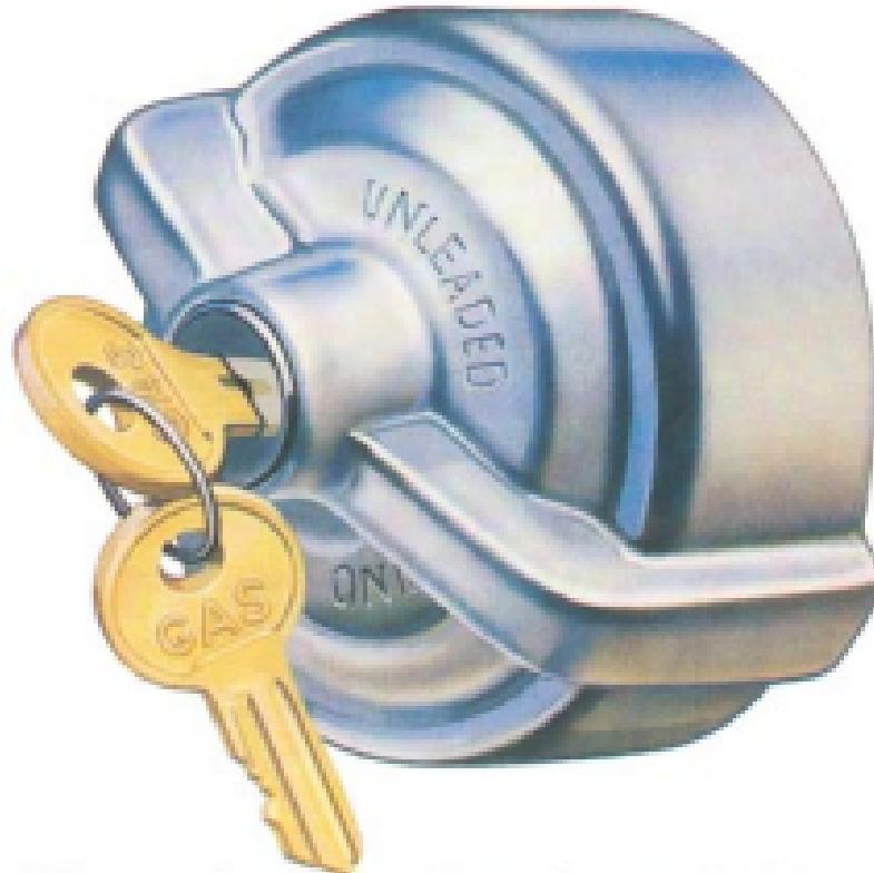
Discourage tampering with your fuel supply with this heavy-duty locking gas cap. It features a sliding key shutter to help keep out moisture, first-quality lock cylinders and comes with two keys.
