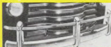
Truck Grille Guard —Protects the truck grille, front fenders and head lamps from damage. 3000 Series type shown. Heavy-duty type also available.
