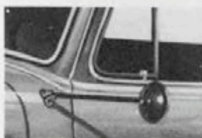
Rear-View Mirrors —Long or short brackets for left-hand or right-hand mounting.
