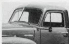
De Luxe Cab —Rear corner windows, bright metal windshield and window reveals, garnish moldings, driver's arm rest, right-hand sunshade and seat back trim panel. Chrome radiator grille.
