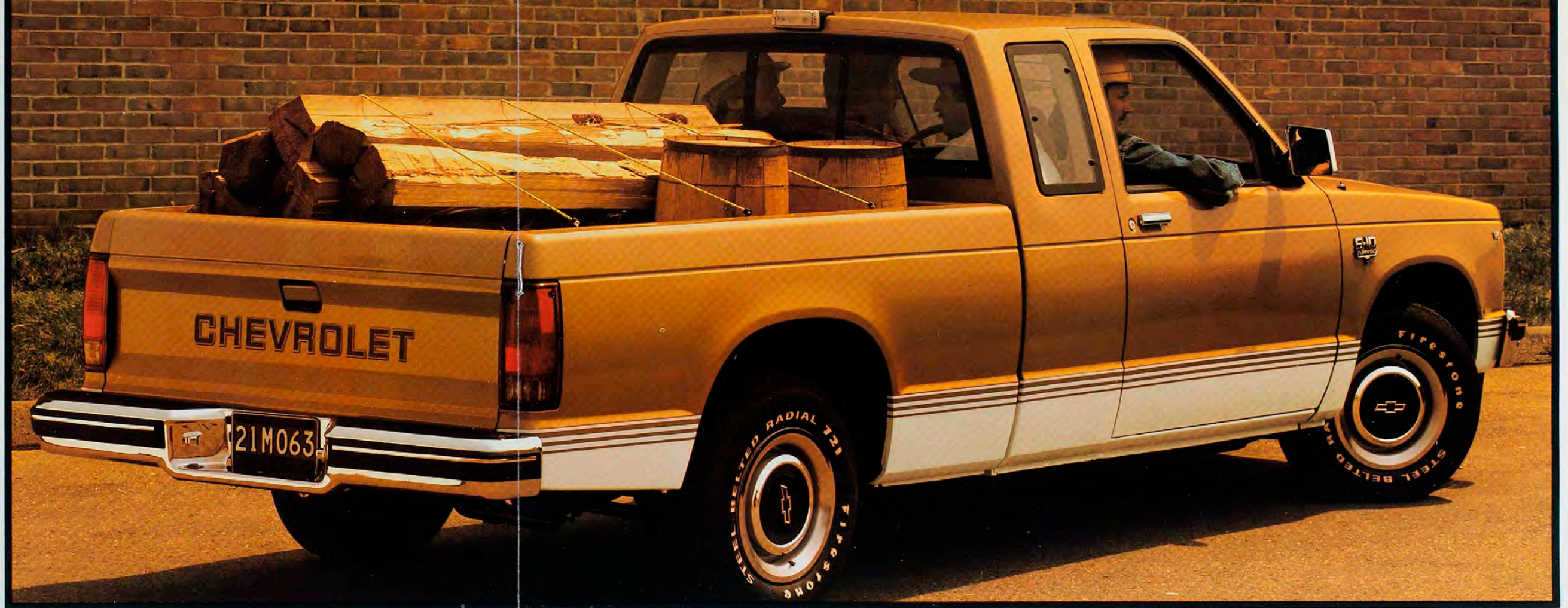
S-10 Maxi-Cab offers optional payloads up to 1500 lbs. (including passengers and cargo).
