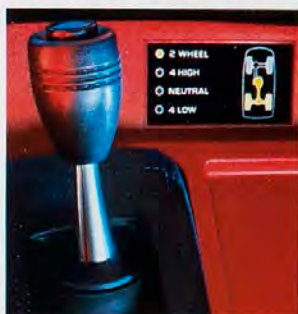
A lighted 4x4 console display in the cab indicates the driving mode with every shift of gears.
