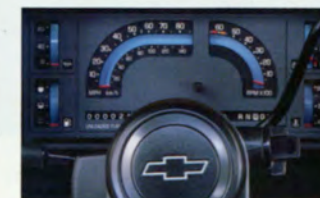
Tahoe instrument cluster, including voltmeter, oil pressure and engine temperature gages and trip odometer.
