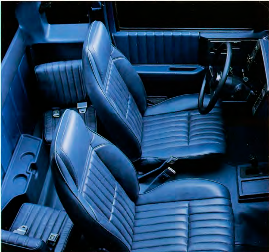
The Maxi-Cab has a longer-than-standard wheelbase (122.9 inches). Optional front bucket seats and rear jump seats in an S-10 Maxi-Cab provide room for four passengers. Rear jump seats fold up and out of the way, providing 13.7 cu. ft. of cargo space behind the buckets. Optional Tahoe trim shown.
