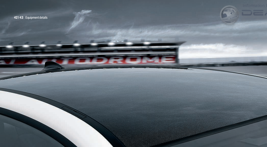
The BMW M3 Coupe's carbon-fiber roof.
