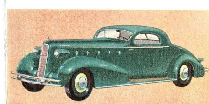
The narrow radiator grill—the streamlined head lamps and supports—the filleting of fender to radiator casing—all contribute to the striking new beauty of the 1934 La Salle. These details have a practical side, too, as their scientific aerodynamic design reduces wind resistance.
