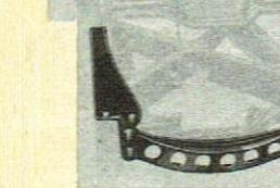
The Fleetwood body on La Salle is sturdily built with a hardwood frame covered with steel panels welded together. The front cowl is strongly reinforced and the roof is of slat and bow construction securely fastened together to provide unusual strength.
