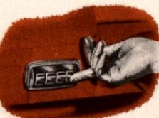
POWER WINDOWS: a new high in convenience, a new note in luxury. You operate all windows electrically—the master control switch for all windows is to the left of the driver and there is an individual switch beneath each window. No special battery or generator needed.
