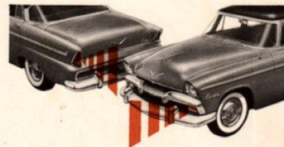
Flashing lights in front and rear tell other drivers your intention when you are turning either right or left. Operated by a single control on the steering column, these dependable turn indicators cancel automatically when the turn is completed.
