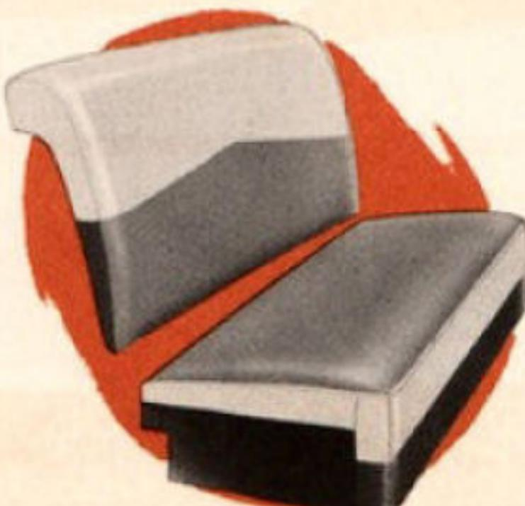
Removable seats, in two easily-handled sections, are available to add more seating area in the Plymouth Business Coupe. They're easily installed to seat three comfortably; easily stored when the extra cargo space is desired. Similar seat sections are available for the Four-Door Suburbans.
