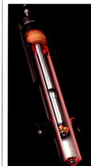
Deflected-disc valving in the shock absorbers is the heart of Buick's Dynaride suspension.
