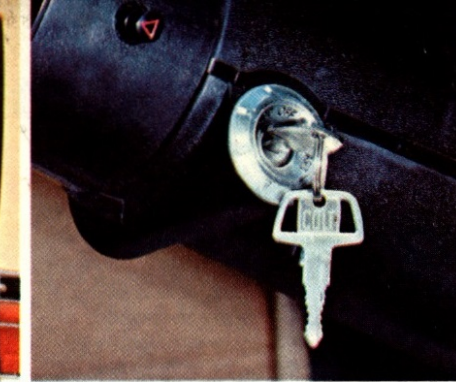
Ignition switch and steering wheel lock. Column has adjustable feature.
