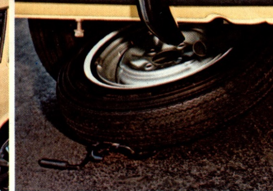
For added cargo space the spare tire is mounted under the rear of the body. Has added feature of anti-theft lock.
