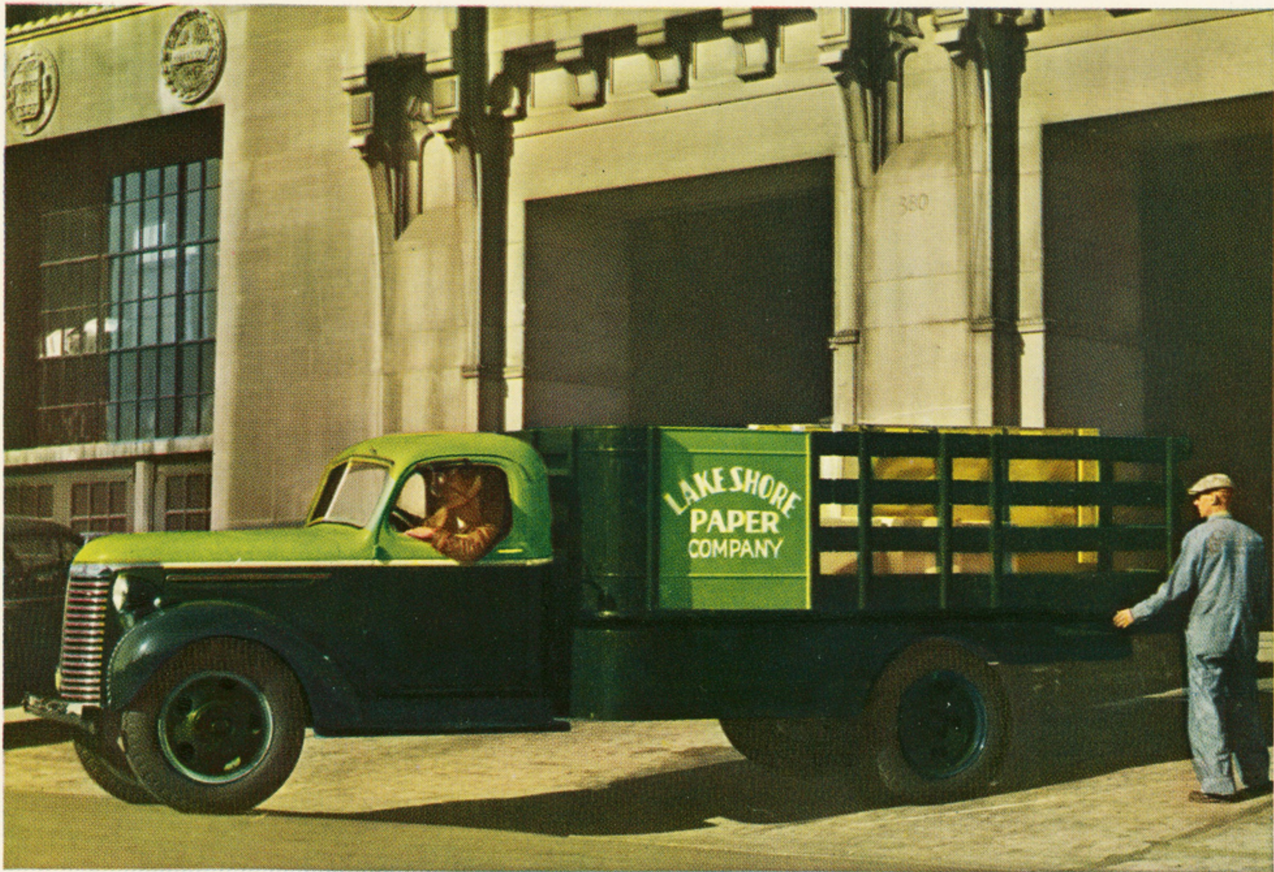
CHEVROLET HEAVY-DUTY DELUXE STAKE TRUCK — 1½-Ton Capacity 158½-Inch Wheelbase. Load Space: 141½ inches long, 80¾ inches wide, 38½ inches high
