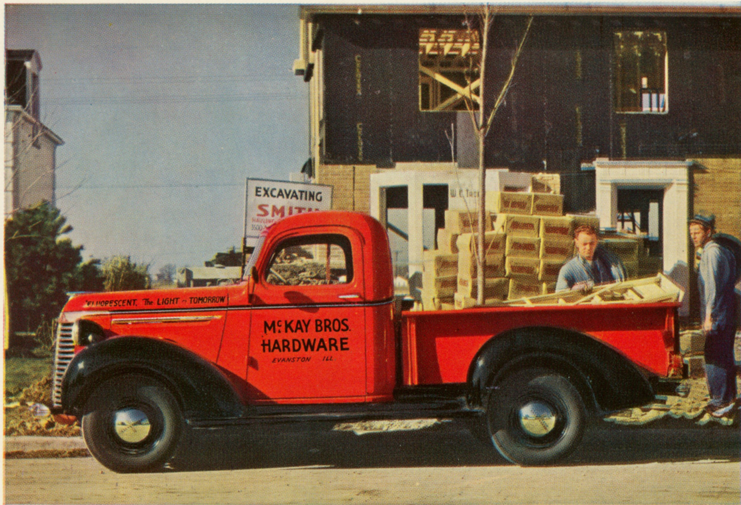
CHEVROLET LIGHT DELIVERY PICKUP TRUCK — Half-Ton Capacity 113½-Inch Wheelbase. Load Space: 78 inches long, 48½ inches wide, 16¼-inch sides
