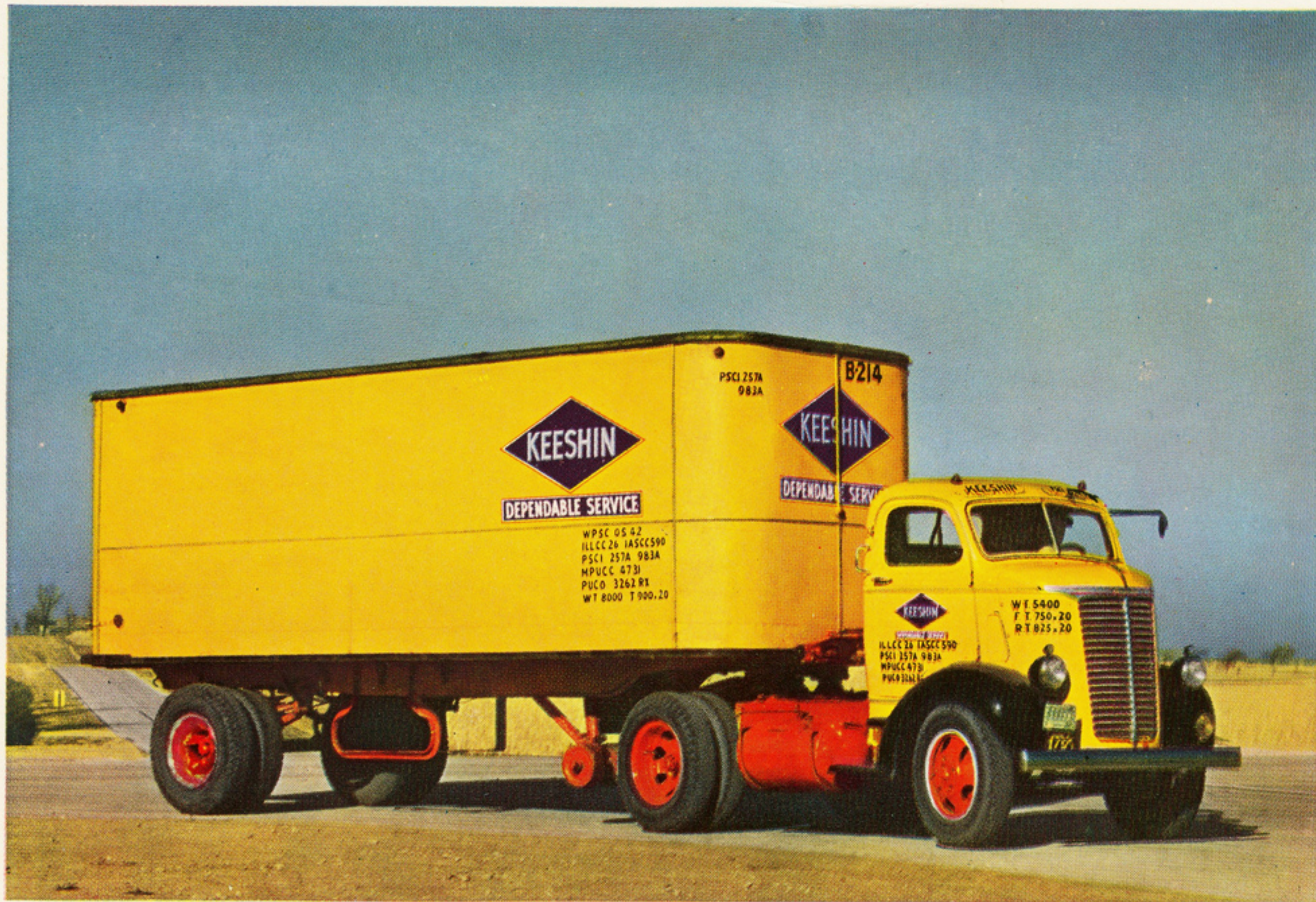
CHEVROLET HEAVY-DUTY CAB-OVER-ENGINE CHASSIS — 107 5 / 8 -Inch Wheelbase For tractor-trailer operations and the mounting of standard and special nine-foot bodies
