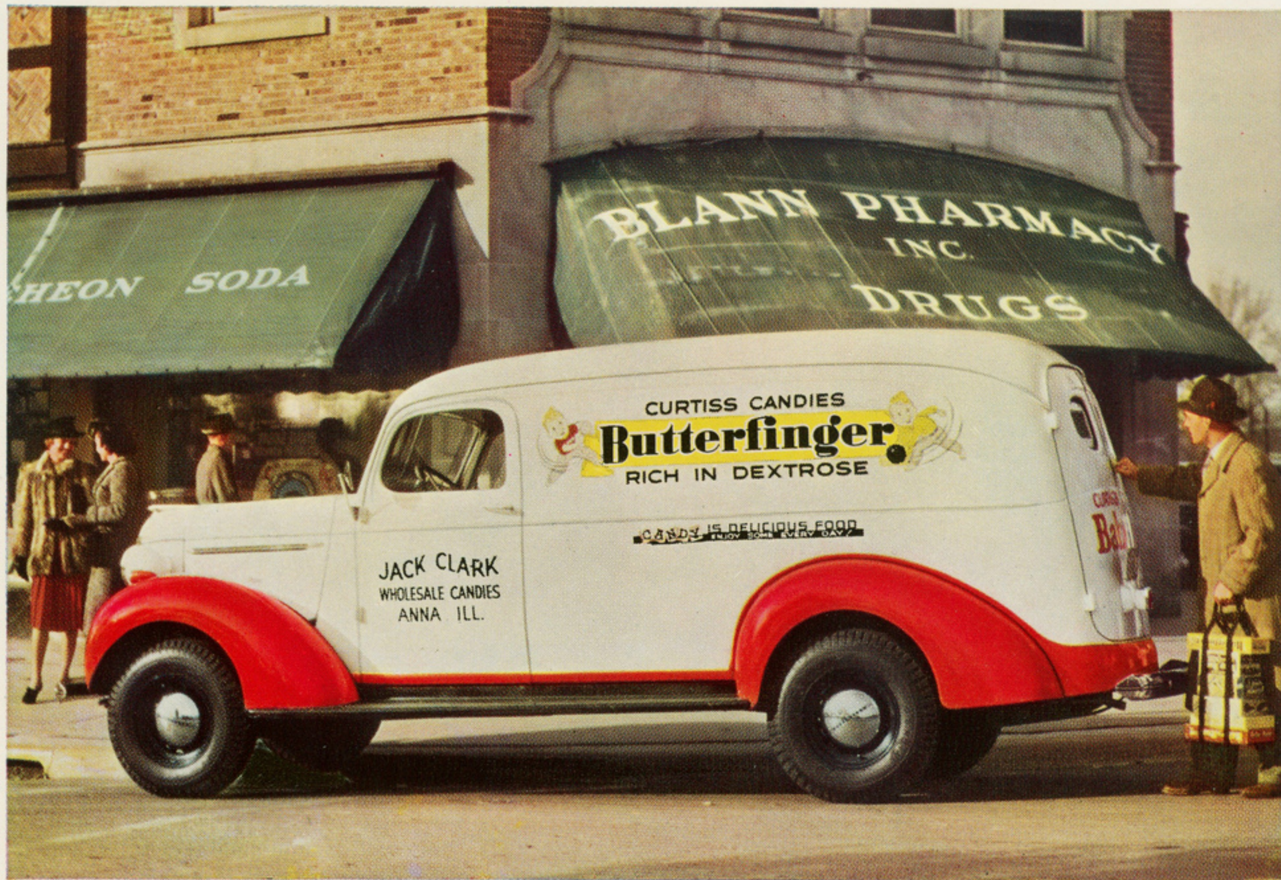
CHEVROLET THREE-QUARTER TON PANEL TRUCK — 123 \frac{3}{4} -Inch Wheelbase Load Space: 96 \frac{11}{16} inches platform length, 57 \frac{1}{2} inches width at belt, 51 inches high
