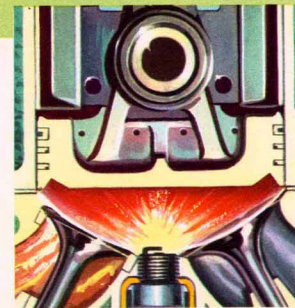
Below is illustrated the Hemispherical Combustion Chamber . . . the heart of the engine and the source of the power-producing efficiency and performance of Chrysler FirePower.
