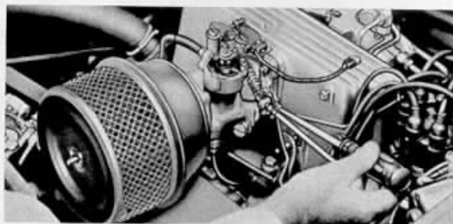
Fuel adjustment screw smooths out idle at proper speed.
