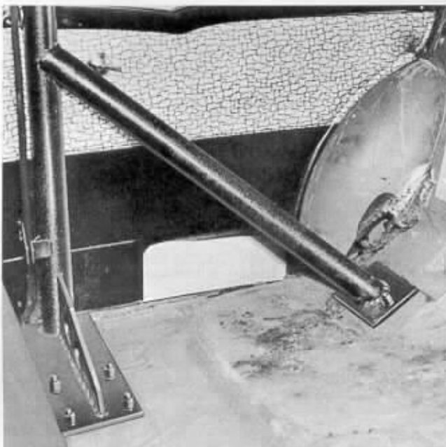
Roll bar must be well braced and properly mounted. Large stanchion feet permit bolting directly to chassis frame.
