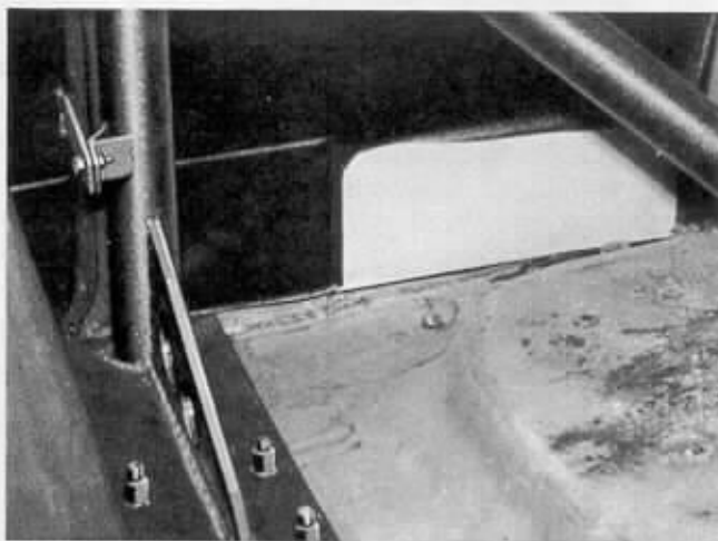
Steel plates and bolts hold right-hand door firmly. Driver enters car through window.
