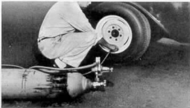
Nitrogen gas minimizes tire pressure buildup. It is available at many tracks, as well as local welding supply houses.
