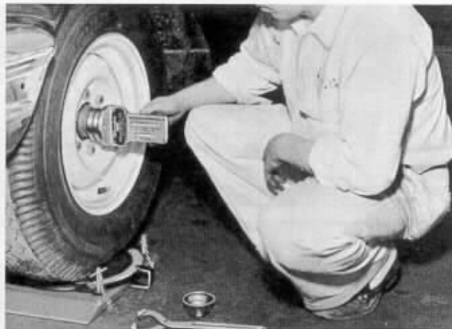
Portable wheel alignment equipment helps determine the proper settings for a specific track.
