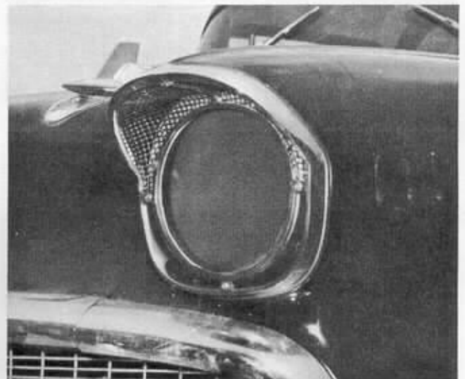
Preferred headlamp closure for 1957 Chevrolet stock cars. Cover fits inside regular headlamp bezel.
