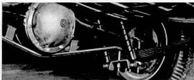
Underside view shows dual shocks mounted at rear wheel. Transverse rod reinforces heavy-duty rear axle.
