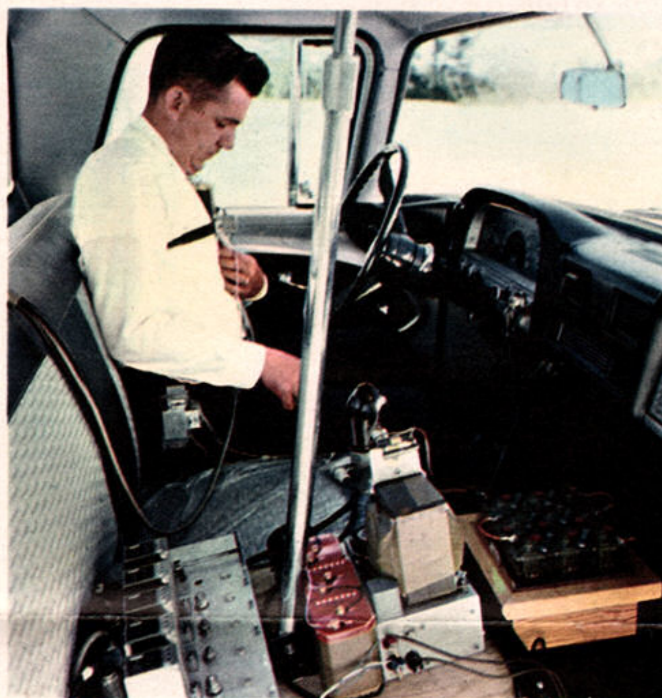
Heavily instrumented test driver prepares to make a ride run in a '60 Chevrolet truck. Strapped on accelerometers register the severity of the jolts he actually feels, in both vertical (bounce) and horizontal (pitch) directions. Accelerometer readings are fed by cable to companion vehicle, where they are tape recorded for later analysis by an electronic computer. The result is an accurate bump-by-bump picture of each test run.
