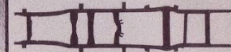
New for Series C10 and C20 models, these ladder-type frames are fabricated of heavier gauge channel side rails spaced 34 inches apart to simplify special body installations. New alligator-jaw crossmembers increase frame resiliency; truck rides softer on rough streets with a frame that "gives" with the bumps.
