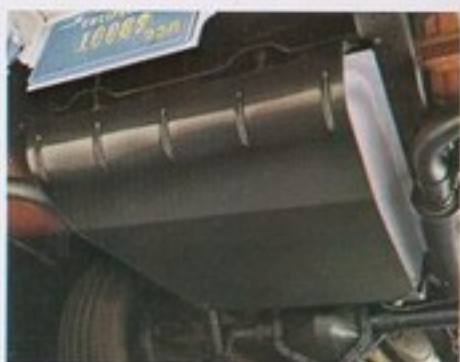
Fuel tank stone shield. 31- and 40-gallon fuel tanks are optional.
