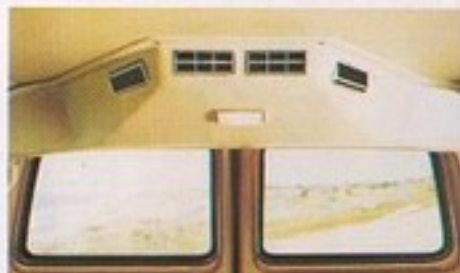
Dual-unit front and rear air conditioning. Each unit can be operated independently.
