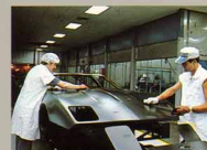
Building the Corvette is a complicated and demanding process, requiring a complex integration of man with machines. A few important phases of the operation are shown here. Clockwise from facing page: A two-stage welder builds the uniframe. Computerized instruments measure body panels to close tolerances. Wet and hand sanding are part of paint application. Point-check inspection helps ensure that body panel assembly meets design intent.
