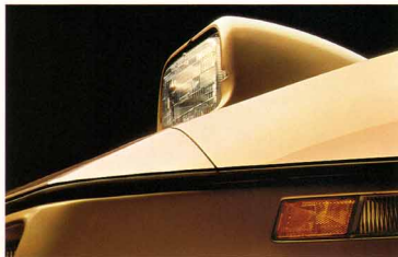
Retractable headlamps flip forward 162.5 degrees from beneath the hood.
