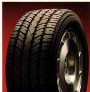
Goodyear Eagle GT P255/50VR-16 unidirectional radial tires.
