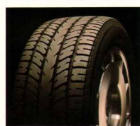
Unidirectional Goodyear Eagle P255/50VR-16 steel-belted radials are mounted on 16" x 8-1/2" aluminum alloy wheels.
