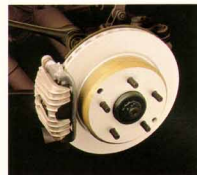
Four-wheel disc brakes feature a large booster for superb modulation, all-temperature brake pads designed to provide consistent performance, and aluminum calipers to reduce unsprung weight.
