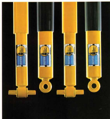
Delco/Bilstein gas-filled shock absorbers contribute to ride and handling.
