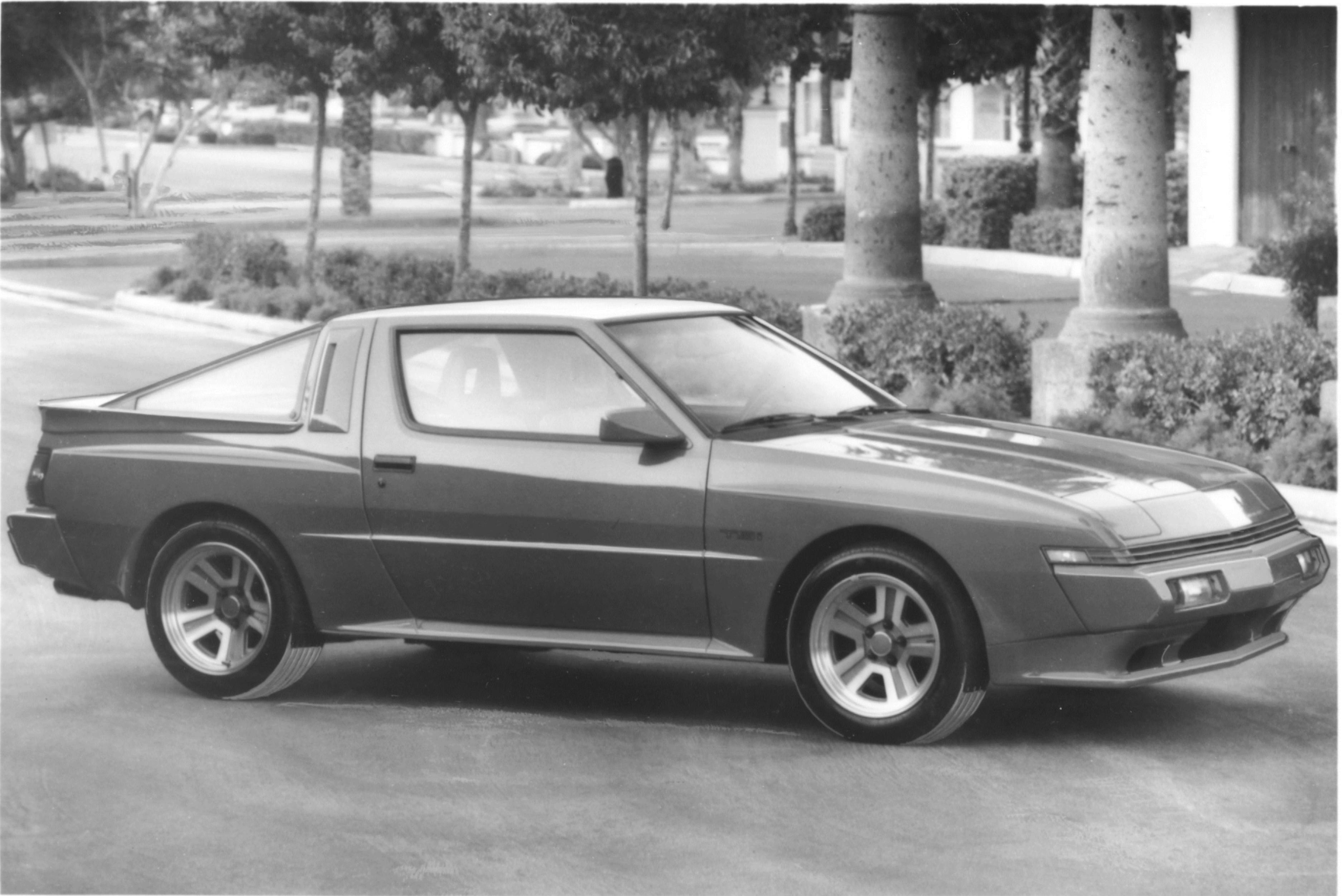
SPORTS SPECIALTY COUPE imported for Chrysler from Mitsubishi is the 1988 Conquest TSi with a solid reputation for appearance, high-tech equipment and performance. Horsepower for its fuel-injected 2.6-liter inter-cooled turbo engine is increased to 188. Extensive standard equipment includes 5-speed manual overdrive transmission, an anti-theft system, anti-lock rear brakes, AM/FM Stereo with cassette and six speakers; power windows, steering and brakes, and speed control.
