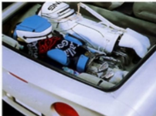
Corvette's new rear-transmission configuration and dual mid-ship mounted fuel tanks allowed engineers to nearly double the available rear storage space for '97. Photo order #97-39COR
