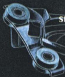
Vibration's Out—A new isolated front sub-frame uses thick rubber "biscuits" to help keep out vibration.
