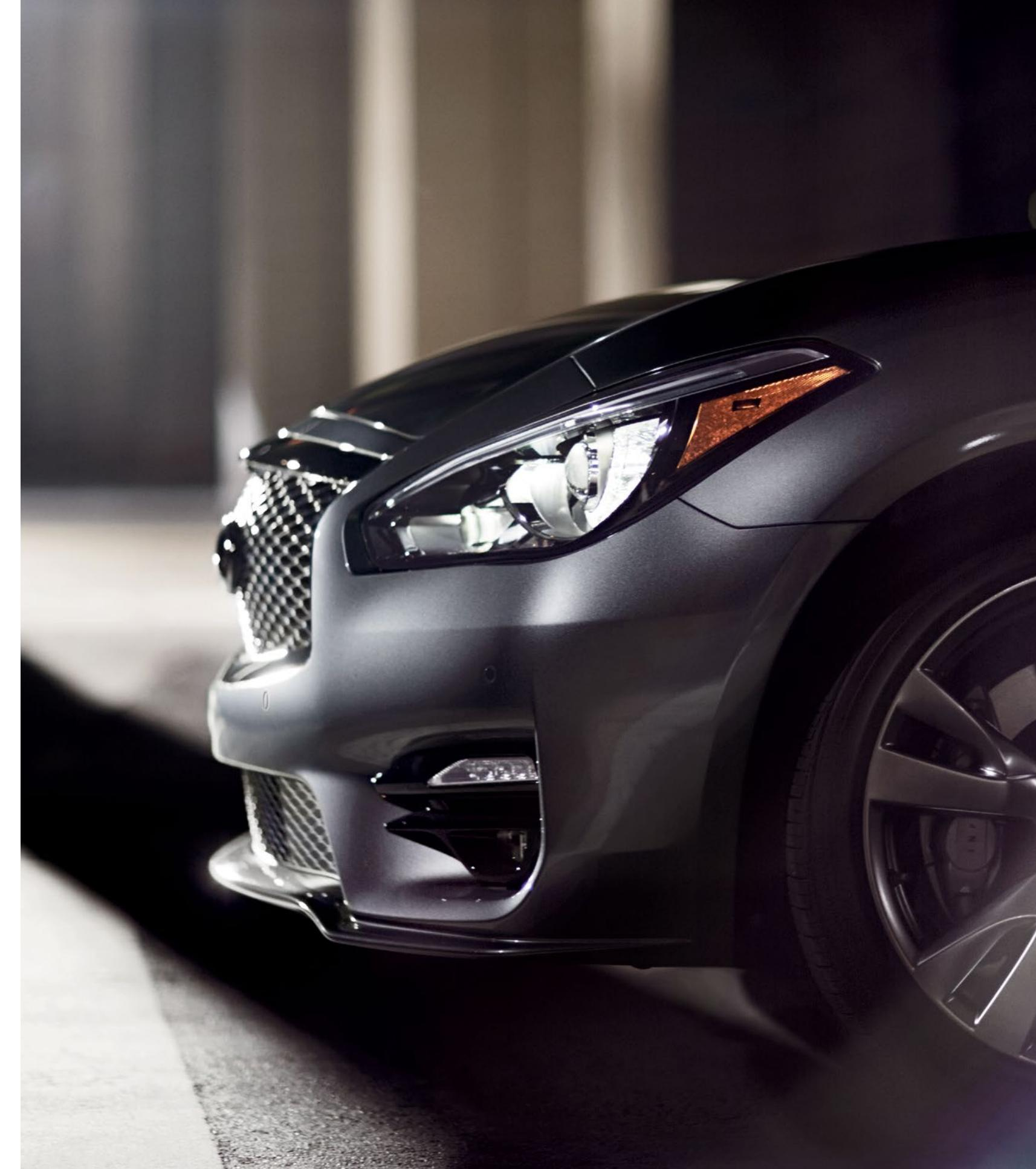
**ATHLETIC STANCE** Large 20-inch alloy wheels not only complement the graceful proportions of the Q70, they are designed to make handling more responsive. The lightweight construction inherently reduces unsprung weight and helps contribute to quicker turn-ins.<sup>1</sup>
