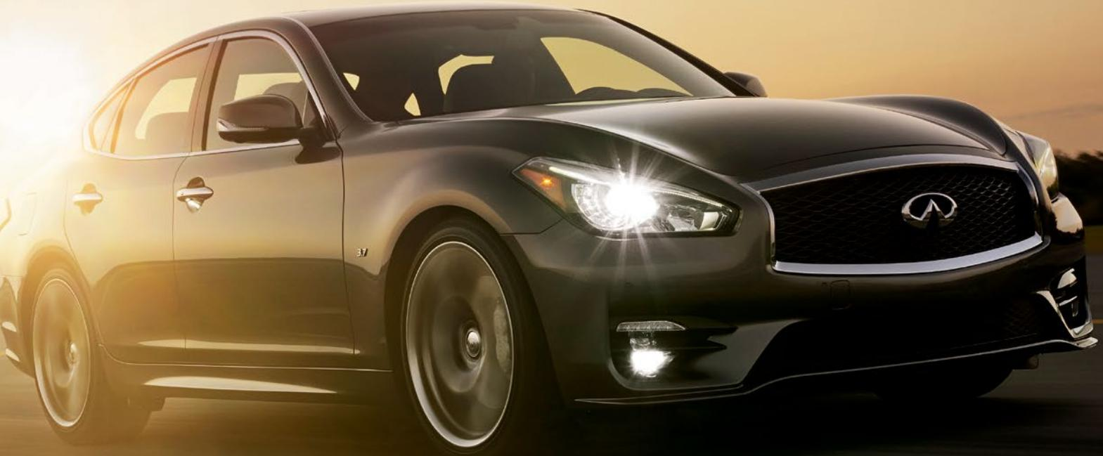
**INTUITIVE TRACTION** Intelligent All-Wheel Drive infinitely adjusts for better traction by sending anywhere from 0 to 50% of the power to the front wheels when you need it, and 100% to the rear wheels for sporty response when you don't. You get AWD traction without sacrificing rear-drive feel.
