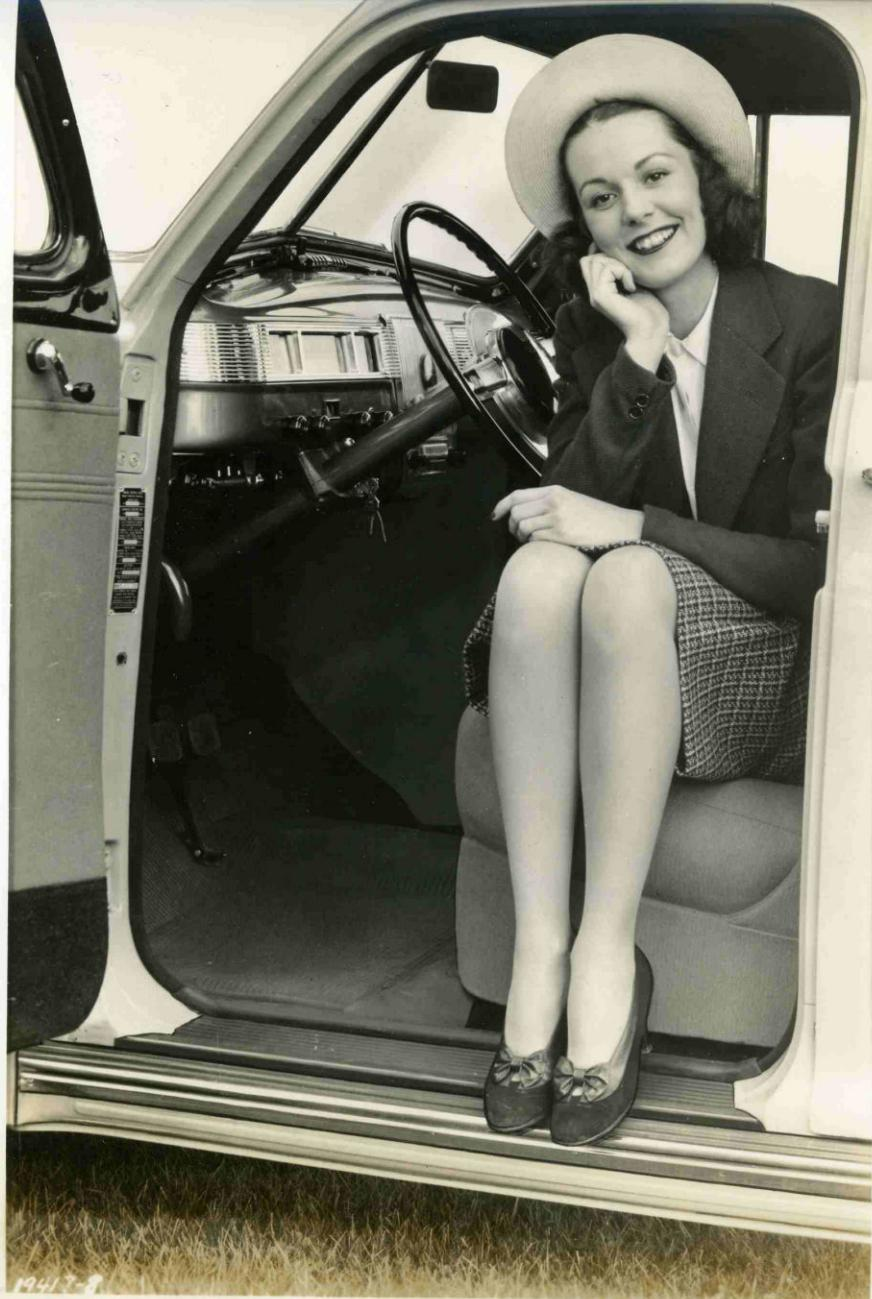
Running boards on the new Nash Ambassadors for 1941 are concealed to provide the cars with greater beauty and greater roominess. They retain their function, however, of safety and convenience. Covered by ribbed rubber, they are only a few inches from the ground, and are flush with the floor level of the new, low "Unitized" steel bodies. The broad doors are completely weather sealed.
