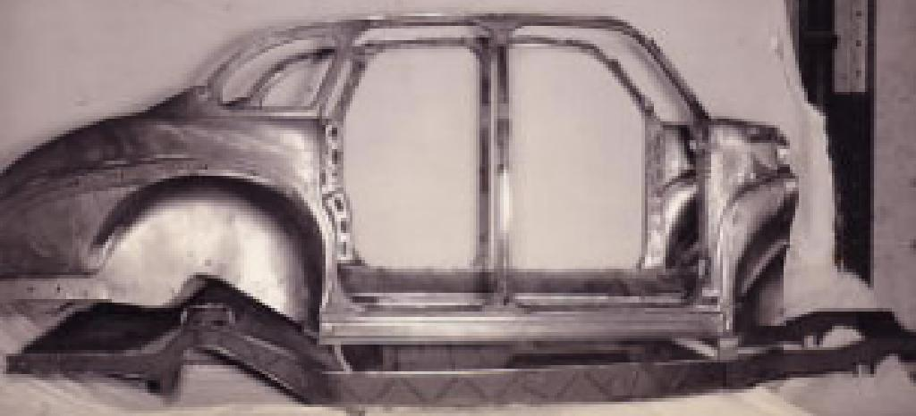
front and front fenders are welded together into a single unit which is stronger, safer and lighter. Bonded, bridge-like girders are used, and the best of light-weight steels are employed. These bodies are built according to the light-weight streamlined trains, it is said. This picture shows the sides and floor before being welded.
