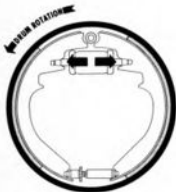
1. Hydraulic pressure forces shoes against drum.
