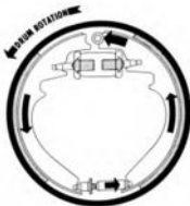
2. Rotating drum moves shoes until rear (Secondary) shoe strikes anchor.
