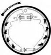
3. Friction between shoes and drum tends to roll both shoes into drum with increased pressure—thus both shoes are self-energized.
