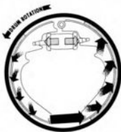
4. Force from front (Primary) shoe is transmitted through the lower link to secondary shoe applying secondary shoe with even greater force.
