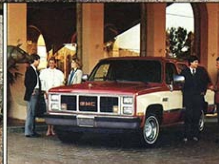
2-WD Suburban with 6.2 Liter V8 truck diesel. Diesel models have standard power steering, power brakes, and heavy-duty electrical and cooling systems.
