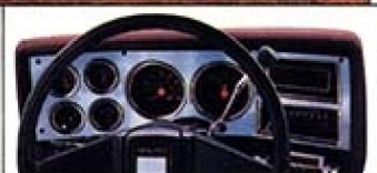
Sierra Classic instrument cluster with needle-type gauges for voltmeter, temperature, and oil pressure
