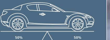
**WEIGHT DISTRIBUTION**, front to rear, significantly impacts handling. So the Mazda RX-8 is designed to maintain an approximate 50:50 weight distribution—regardless of passenger load. Much of the credit for this remarkable feat goes to its rotary engine. Smaller and lighter than a piston engine of comparable power, it also provides the RX-8 with a superb power-to-weight ratio for spirited acceleration. And more cabin space to comfortably enjoy its inspiring performance.
