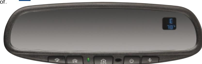
**C. Compass & Outside Temperature Auto-Dimming Mirror**
