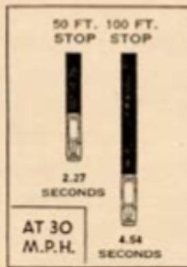
to stop us in twice that distance. How much better it is, under any normal circumstances, to begin to apply the brakes a few seconds earlier and, with gradually increasing pressure, bring our car to an easy stop. As a matter of fact, smooth, gradual stopping, wherever the circumstances permit, is generally taken as a sign of a good driver.
