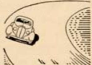
a centrifugal force of only about 156 pounds at 20 miles an hour. But at 30 miles an hour, that force has grown to 360 pounds, and at 60 it is nine times as great as at 20 . . . over fourteen hundred pounds trying its best to push us off the road! The only thing that keeps us on the road in the first place is the friction between our tires and the road. The minute the centrifugal force gets stronger than the force of that friction, off the road we go.
