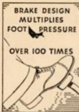
What brakes really do is to convert speed-energy into heat-energy. When we push down on the brake pedal we press the brake lining against the brake drums and this creates friction that changes the energy to heat. When we have changed all the speed energy to heat, then we come to a stop.
