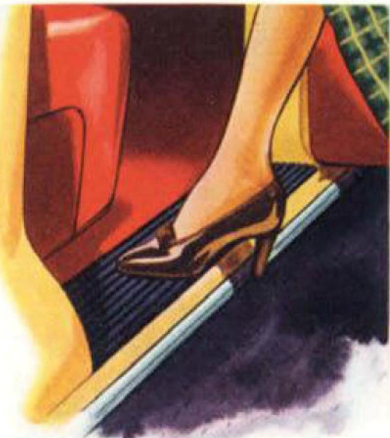
*The running boards are enclosed within the body structure. This greatly increases the fluent beauty of the car's lines, and is a safety feature too. The rubber-covered step remains dry, clean, non-slippery, in all weather.*
