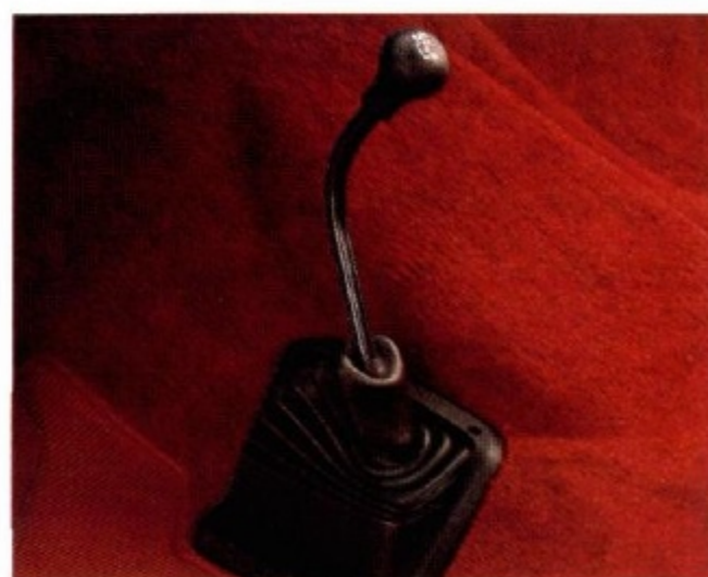
2-speed transfer case includes a neutral tow feature.
