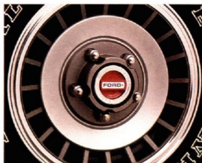
Manual locking hubs are easy to operate. A simple quarter turn is all that's needed to engage or disengage 4-wheel drive.
