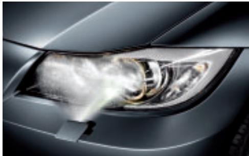
■ **Headlight cleaning system** ensures optimum headlight brightness in all kinds of weather. When the lights are on, the headlights are automatically cleaned in parallel with the windshield. (Available only on the BMW 328xi.)
