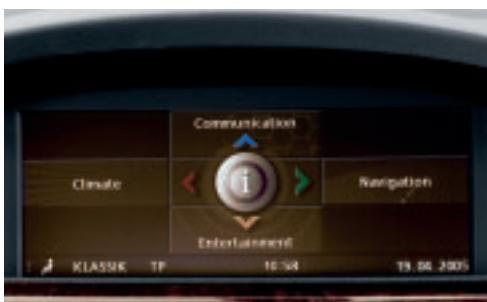
□ **Navigation System Professional**, including DVD drive and iDrive Controller. Destination input via voice control. Directions are given via arrows and a map displayed on an 8.8" monitor.
