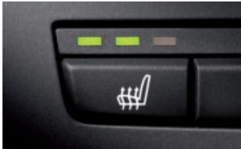
■ **Seat heating** for driver and front passenger (three settings): seat surface, sides and backrest are heated and quickly radiate comfortable warmth. (Optional on the BMW 323i.)
