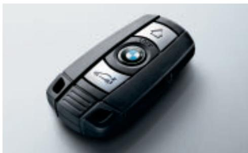
□ **Comfort access system** for opening and locking the vehicle without having to operate the radio remote control. It's enough to have the ignition key in your pocket, briefcase or handbag. In addition, the engine can be started without the need for a key, using only the Start/Stop button. (Available only on the BMW 335i.)
