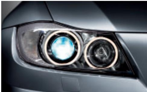
■ **Xenon headlights** for low and high beam, with luminous rings and automatic headlight range control, provide much better illumination of the road ahead at night or in poor visibility. These headlights also feature auto-levelling to adjust for varying passenger and cargo loads. (Available on the BMW 328i/xi and 335i.)
