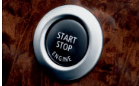
■ **Start/Stop button** for starting the engine. After inserting your ignition key, you can start and stop the engine by pressing this button.
