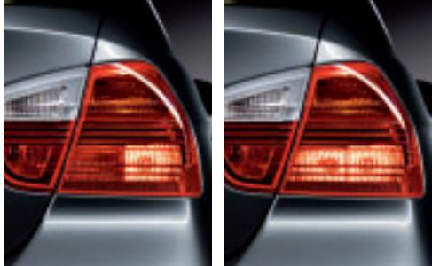
■ **Adaptive Brakelights** help vehicles travelling behind you to evaluate your braking more accurately. In the event of an emergency stop, the illuminated area of the brakelights is increased, so traffic can tell in an instant the difference between a light tap on the brake pedal and a hard stop.
