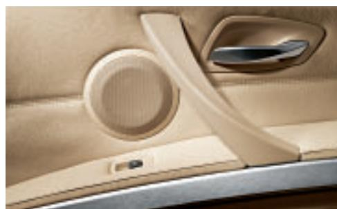
□ **LOGIC7 Sound System** provides truly outstanding sound. 13 loudspeakers and the adjustable surround function create a luxurious soundscape all around you. The central bass concept uses two subwoofers beneath the front seats to reproduce an authentic bass sound.
