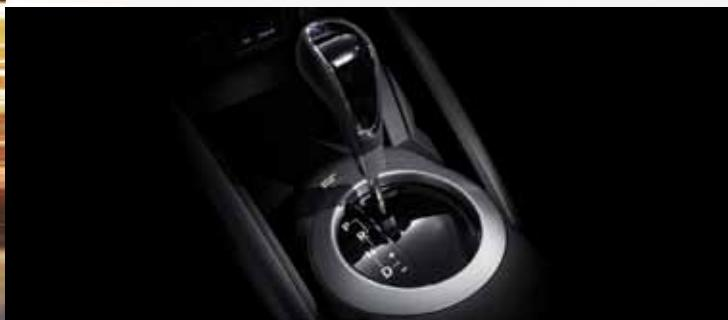
The Veloster is the first Hyundai to feature an advanced Dual Clutch Transmission (DCT). Appropriately named EcoShift DCT, it takes the benefits of a manual transmission, low fuel consumption and peppy performance, and blends them with automatic transmission benefits, such as a comfortable ride and smooth shifts. The Veloster is also available with optional paddle shifters to really take advantage of the performance of the EcoShift DCT. It's one serious piece of machinery.
