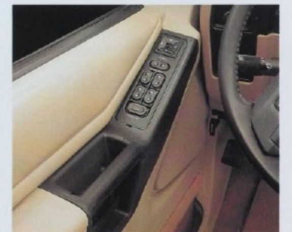
Features of the optional power equipment group (power door locks, windows, and electric remote-control mirrors) are located on a special ergonomic door-mounted panel. Tactile controls, easily identified by touch alone, are designed with a "bump" at one end ("on") and a "dimple" at the other end ("off").
