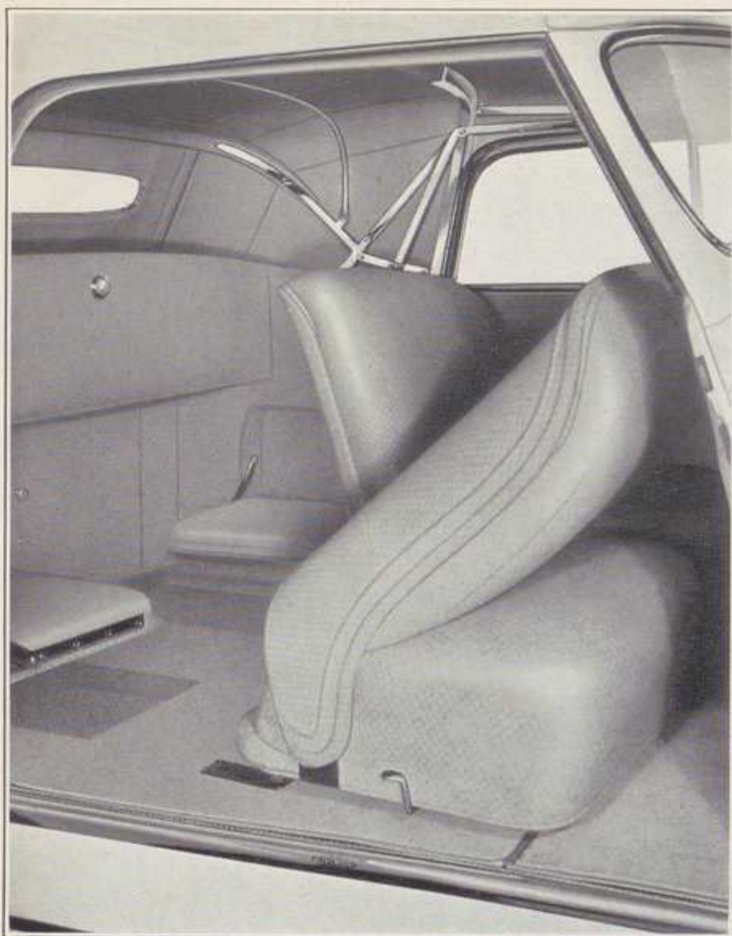
The inside auxiliary seats provided in the Fleetwood Convertible fold into the side walls when not in use completely concealed, providing a large carrying space behind front seats. A compartment accessible from interior of body is provided behind the front compartment.
