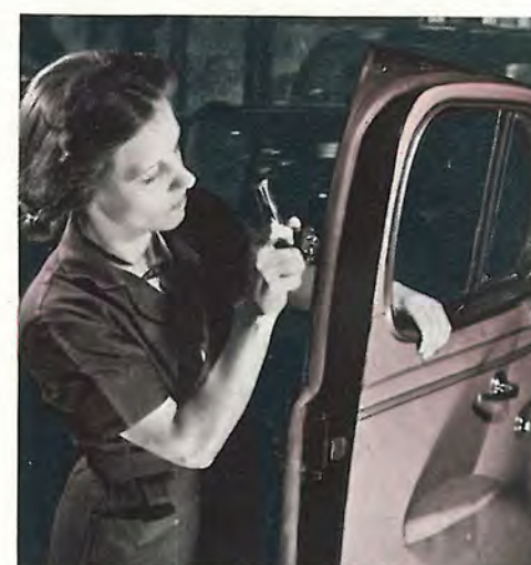
Body building, too, with such special processes as painting door and trunk edges—most difficult operations—are Packard's own.
