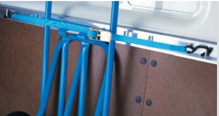
Side cargo storage rail Allows loads to be easily and securely lashed. (Option, load strap not supplied, shown with load compartment trim board)
