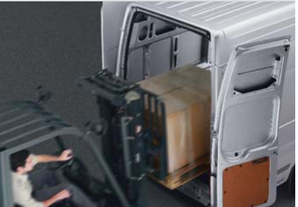
Rear doors. 180° opening unglazed rear (Standard) 256° opening doors with magnetic retainers (Option. Standard on 'Jumbo')
