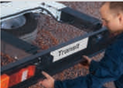
Detachable rear member simplifies bodybuilding applications.
