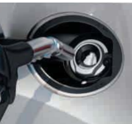
Ford Easy-Fuel capless refuelling system (Standard)
