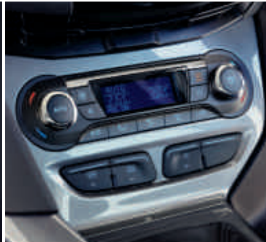
Dual-zone Electronic Automatic Temperature Control (DEATC) (Standard)
