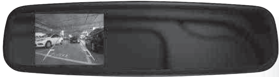
Rear-view camera Select reverse and the image from the rear-view camera comes on automatically in the rear-view mirror. Marker lines overlaid on the camera image indicate where the vehicle is heading. (Option)
