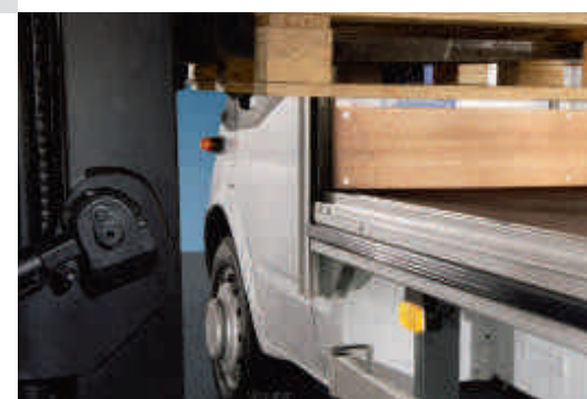
Bump strip Optional bump strip helps reduce damage from fork trucks.
