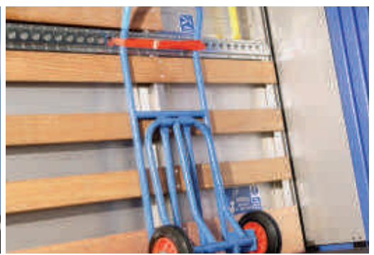
Load-loc rail Optional bulkhead load-loc rail and additional laths, 6 fitted as standard.
