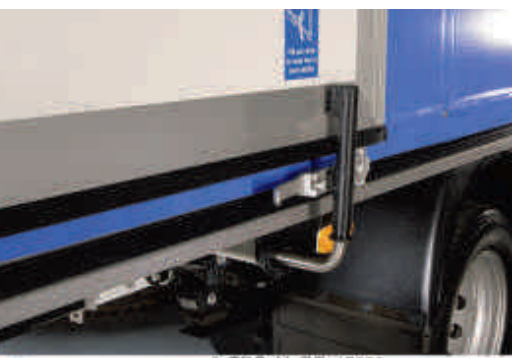
Telescopic rear door retainers Hold doors safely in the 270-degree position. Brolly handle retainers rotate and stow under the load deck when not in use.
