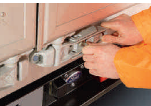
Lockable rear door handle Lockable rear door handle with top and bottom latches.
