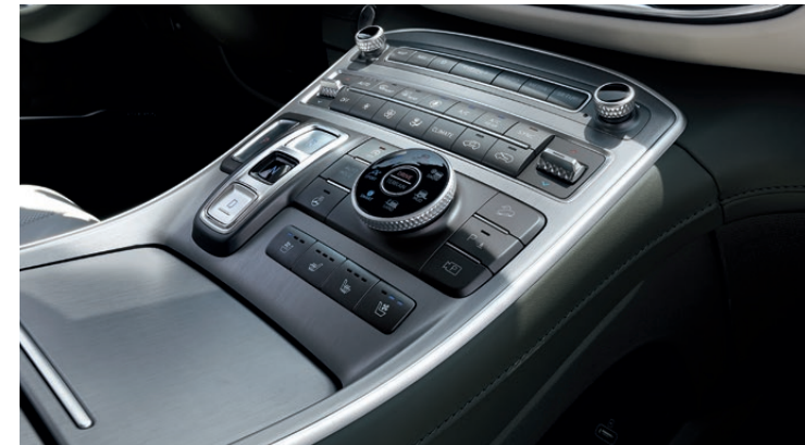
Floating high console with shift-by-wire transmission standard across all trim levels. Aluminum finish standard with Luxury pack.
