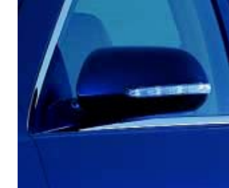
Door mirrors also feature indicator repeaters for enhanced visibility.
