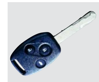
To allow best use of the power tail gate, the control is incorporated in the latest design ignition key.
