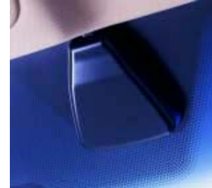
This unit behind the rear-view mirror activates the rain-sensing wiper system, which automatically adjusts the wiper speed according to rain intensity, and can be fine-tuned using a control on the stalk. Standard on Executive models.
