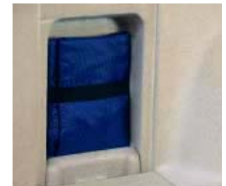
A removable panel in the side wall of the cargo area conceals a small storage compartment, with straps to secure a first-aid kit or other items.
