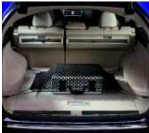
This neat tie-down cargo net prevents small objects from slipping in the boot, improving safety and convenience and avoiding possible damage to internal fittings and finish. A tie-down belt is also available to secure larger items.
