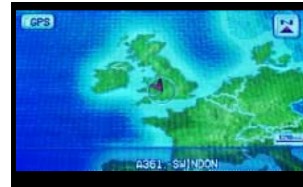
The Satellite Navigation system uses pan-european DVD based mapping software and GPS (Global Positioning System) and can determine your exact location.
