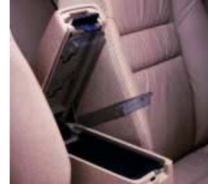
The armrest lifts to reveal a shallow trinkets tray, which can be raised using a separate lever to open up the deeper storage box underneath.
