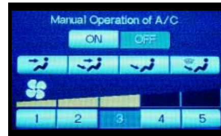
The Satellite Navigation screen also controls the air conditioning.
