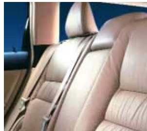
The three rear head restraints and three-point seatbelts are fully integrated into the seat back as part of the Tourer's unique One Motion rear seat folding mechanism.
