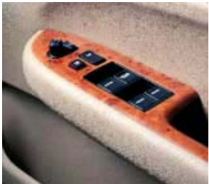
Controls for electric door mirrors and front and rear windows as well as the security lock are neatly mounted in the driver's door handle unit.
