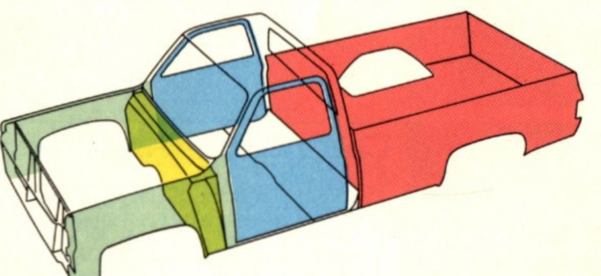
final priming. Primer also is baked on the inner surfaces of the outer front door panels before forming and final priming. Pickup box steel floor, sidewalls, front panel and tailgate are totally immersed in primer and electrically charged—drawing paint into hidden seams and crevices for added corrosion protection.
