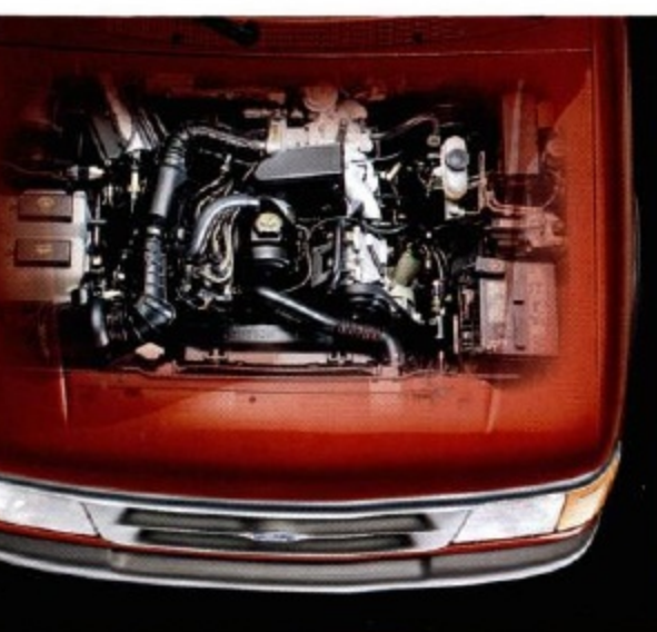
The 2.3-liter I-4 gets a big boost in Ranger for 1995. Its new intake manifold and new cylinder head design for enhanced air flow are among the improvements that give this engine higher performance.
