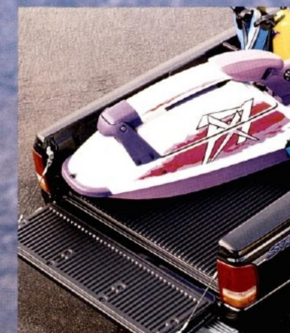
High-density bedliner helps guard against damage and includes a protective tailgate panel.
